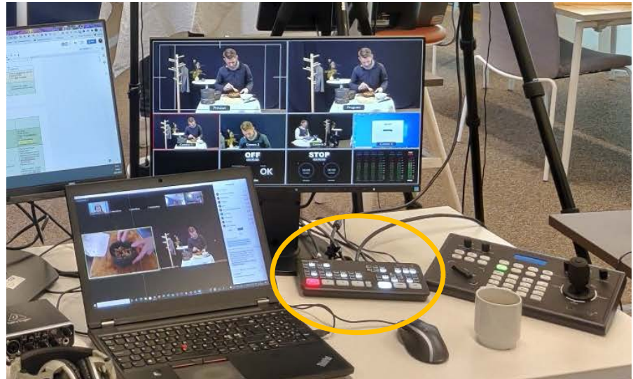
Figure 8: Producer table the videomixer in the middle and the multiview from the mixer on the screen.
